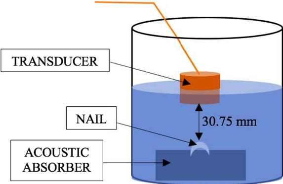
**Fig 3. Cavitation Experimental Design A) With Nail B) Without Nail:** Cavitation Experiment experimental design. Acoustic Absorber (+/- Nail) was placed in water bath at set distance from an ultrasound transducer. The PCD was set to intersect the path of ultrasound.
