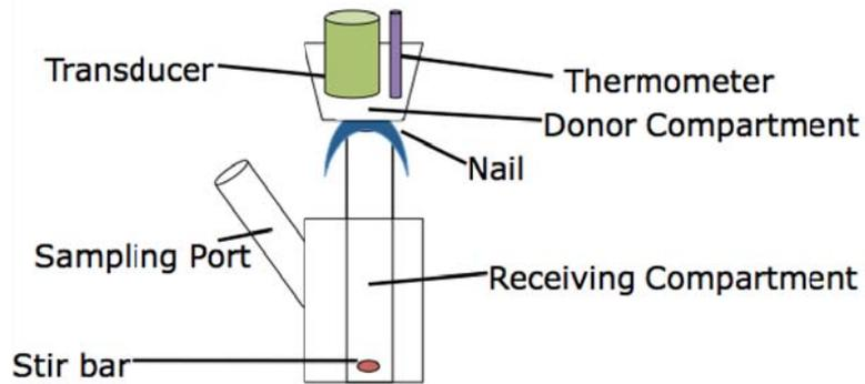
**Fig 2. Luminosity Setup:** Luminosity Experiment experimental design. Nail was sonicated in blue dye at set distance from the ultrasound transducer. Nail was placed on acoustic absorber.
