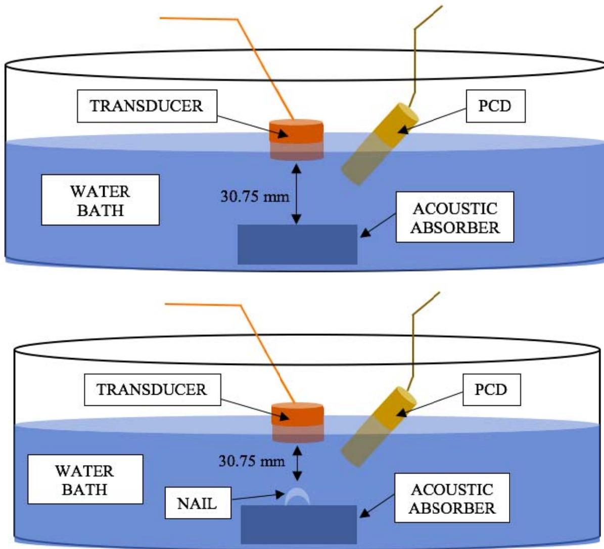
**Fig 4. Streaming Setup:** Streaming Experiment experimental setup. Nail was first placed in saline at set distance from ultrasound transducer. Nail was then moved into blue dye for set amount of time with no sonication.
