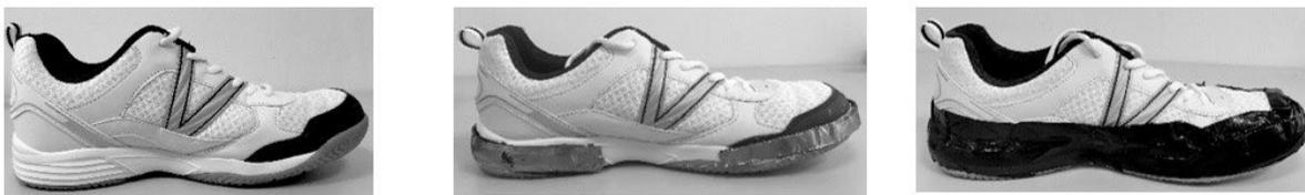
**Figure 1.** Procedure of weighting shoe sample in the experiment. A, Indoor running shoe (control shoe). B, Lead tape added to fore and rear parts. C, Concealed with the black tape.
